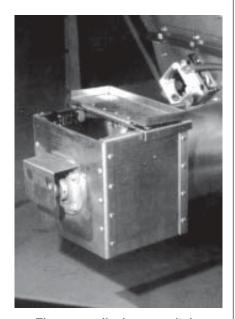
The auger discharge switch.
